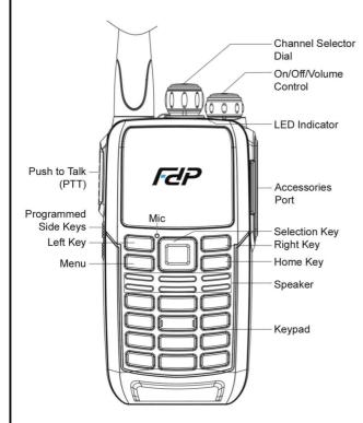
The FDP DMR800 5W UHF Handheld Transceiver is primarily intended for the Land Mobile Service, both in DMR and analogue, covering 400-480Mhz. The radio can also be used on the 70cm Amateur Radio Band by licensed ham radio operators.
