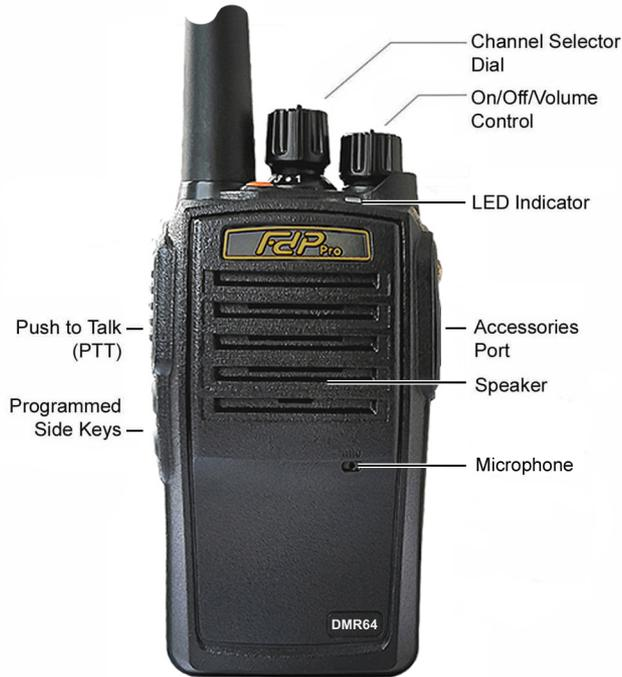
The FDP Pro DMR64 5W UHF Handheld Transceiver is primarily intended for the Land Mobile Service, both in DMR and analogue, covering 400-480Mhz. The radio can also be used on the 70cm Amateur Radio Band by licensed ham radio operators.
